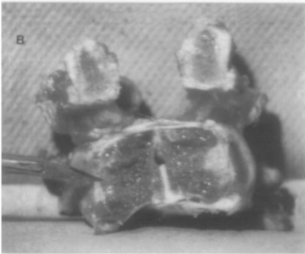
Fig. 4. End plate fracture (A) and intrusion of nuclear material (shown at the tip of the scalpal) into the vertebral body (B) from compressive loading of a spine in a neutral posture. These are porcine specimens from our laboratory.
